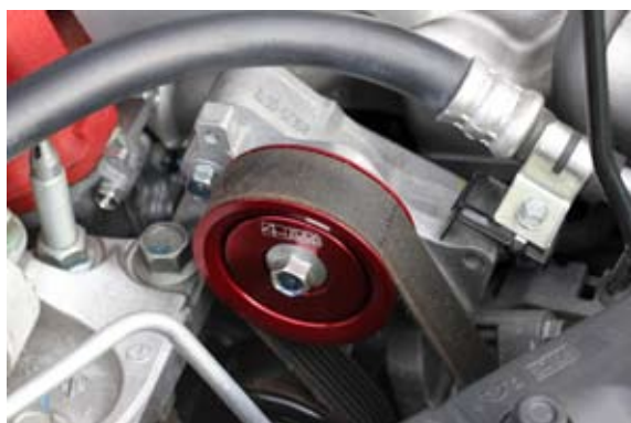
■ Installed Idler pulley.
