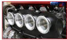
Image of the 33mm long trumpet. Tank depth limits the trumpet length to 33mm.
