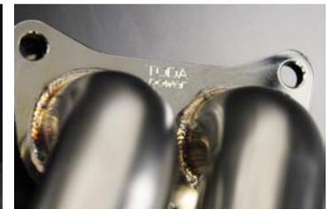
TOYOTA 86/ SUBARU BRZ Exhaust Manifold (less catalyzer)
