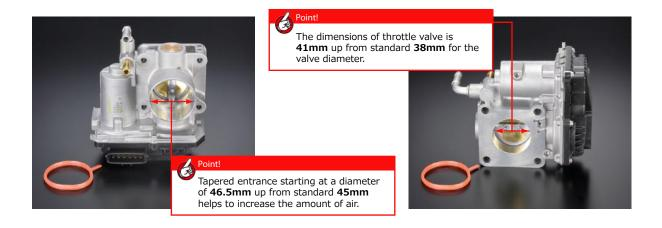
Increasing the diameter of the throttle and in combination with a tapered entrance helps to increase the amount of air the engine can breathe, giving improved performance. All parts are new. No trade-in is required so you get more performance and a new throttle assembly. By using with TODA light weight flywheel and light weight front pulley kit, you will experience a more sportier S660.
